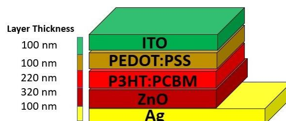
Fig. 11. Simulated Organic Solar cell with layer Thickness
